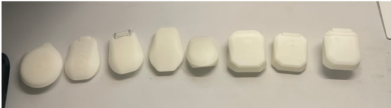
Figure 7.5: 3D printed design iteration
